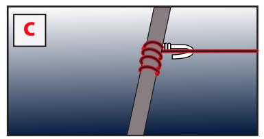
WIND CABLE AROUND OBJECT AND TIGHTEN SECURING THE HOOK.
